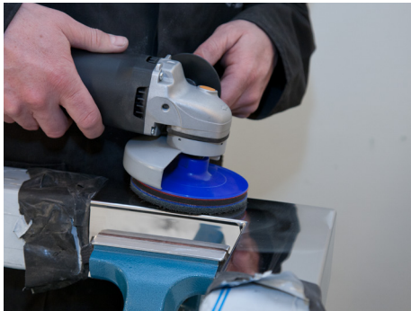
Prepolishing: ideal last step before mirror polishing.
