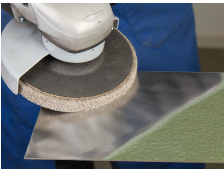
Removing varnish, coatings and rust without affecting the geometry.
