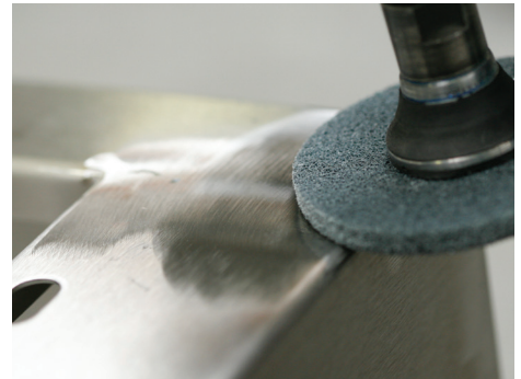
Improving surface roughness. Controlling the Ra value.
