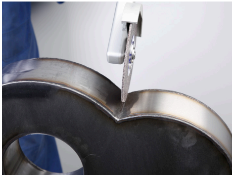
Removing TIG welds.
