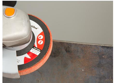
Breaking angles, deburring and rounding.
