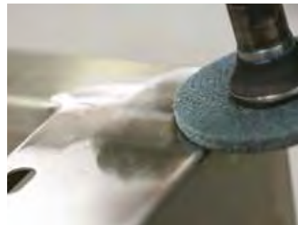
Improving surface roughness. Controlling the Ra value.
