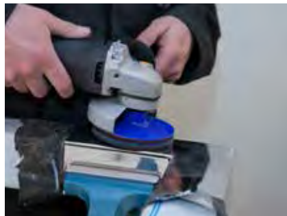
Prepolishing: ideal last step before mirror polishing.
