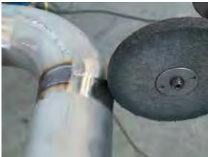
Removing welding discoloration.
