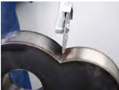
Removing TIG welds.
